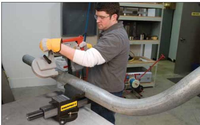
◀ Enerpac BV5 Hydraulic Bench Vise with hands-free XA11G Foot Pump makes work with a large heavy piece into a one person job.
